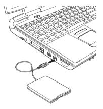
Figure 4-3 Connecting the USB diskette drive
